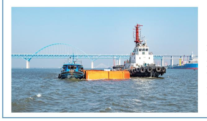
On 16 April, the 1st section of collision protection facility of pier No.26 of Shanghai-Nantong Yangtze River Bridge was transported from the port of Nantong Jiaolong Heavy Industries to the installation site. As protection facilities have been completed one by one, the bridge's water work will be completed.
