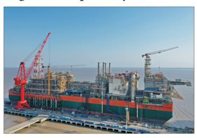
A few days ago, Qidong COSCO shipping and marine engineering N999 FPSO project engine room power system test was started. N999 FPSO is the first floating production, storage and offloading ship built by Chinese shipbuilding enterprise for African project. The ship is 270 m long, 54 m wide, 31.5 deep. It has functions including oil and gas production, process, storage, offloading and transport, and mooring positioning. After it is completed, it will go to Africa for operation.
