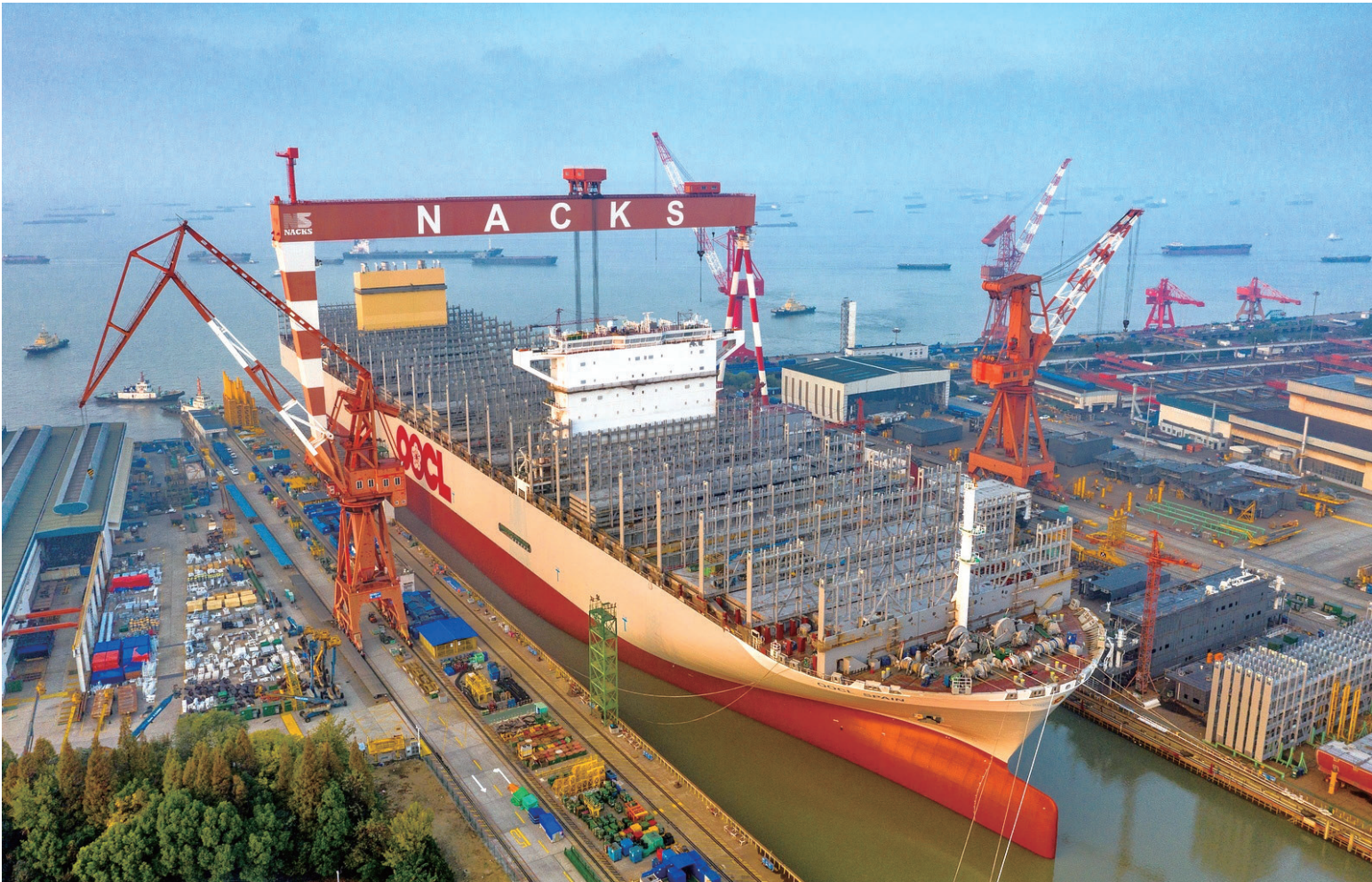
On 15 November morning, a super large ship which can carry 24000 standard containers was launched successfully at Nantong COSCO KHI ship engineering Co., Ltd. The ship is 399.99 m long, 61.3 m wide. The deck area is equivalent to 3.5 standard football fields. It is one of the container ships with largest scale and most container lots in the world.
