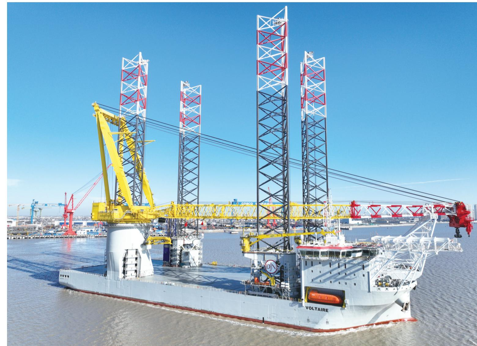
The first 3000 ton self lifting self propelled wind power installation ship in the world
